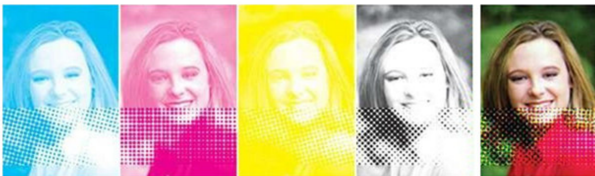
Cyan, magenta, yellow, and black (CMYK) separations with halftone. (Exaggerated to show details.)
